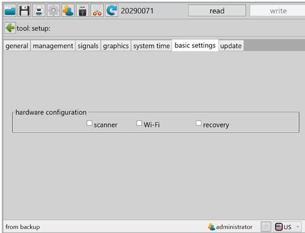
Under „basic settings“ accessories can be activated, such as Wi-Fi and barcode scanner as well as the recovery function.
