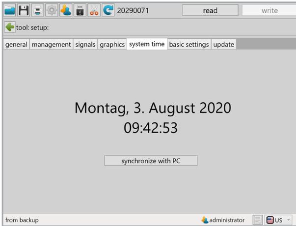
In the system time tab the real time clock (RTC) can be synchronised with the time of the computer connected.
