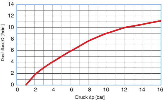
CHECK VALVE® Flusskurve – unscreened BF660080024100; T = 50 °C, Hydrauliköl HLP46
