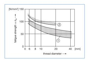
For hot-dip galvanized screws the fatigue strength is about 20% lower than for screws hardened and tempered at the end of the manufacturing process.
