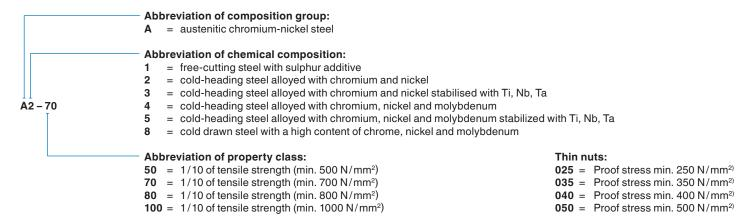
Screws with reduced load bearing capacity due to the head or shaft design that can be subjected to a tensile test are now labeled with the property class by the supplementary number 0. For example 050, 070, 080, 0100.
