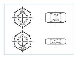
If the nuts of grades A2 and A4 are marked with grooves and the property class is not specified, then the property class 50 of 025 applies.
