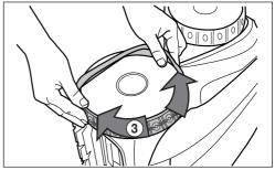
Figure 27. Work the Tyre On Around the Wheel
