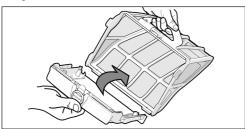
Figure 14. Separate Vanister from Support
