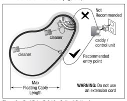
Figure 6. Pool Entry Point for Optimal Patterning
