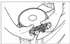
Figure 23. Pull the Old Tyre Over the Wheel
