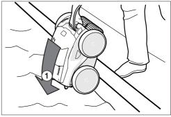
Figure 4. Submerge the Cleaner Vertically
