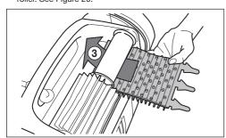
Figure 20. Install the New Brush
