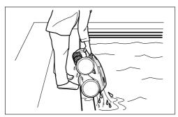
Figure 8. Keep Cleaner Vertical to Drain Water
