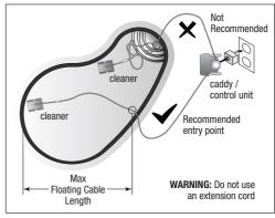
Figure 7. Optimal Entry Point in Pool
