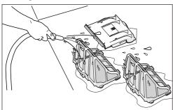
Figure 16. Wash Filter Canister
