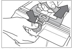
Figure 13. Open Filter Canister Assembly
