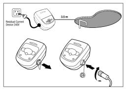
Figure 3. Connect/Disconnect the Floating Cable
