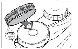
Figure 25. Tyre Replacement Orientation
