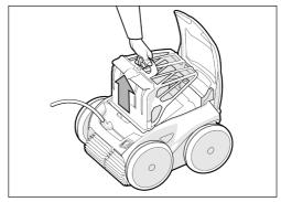
Figure 12. Remove Filter Canister Assembly
