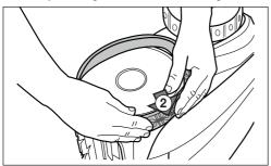
Figure 26. Start on One Side of the Tyre
