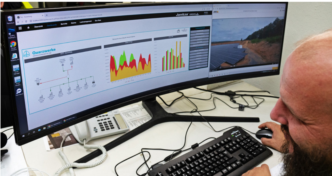
The GridVis® provides a complete overview of the entire plant from the office
