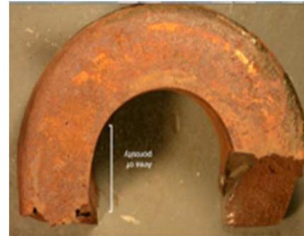
Anchor crown broken
