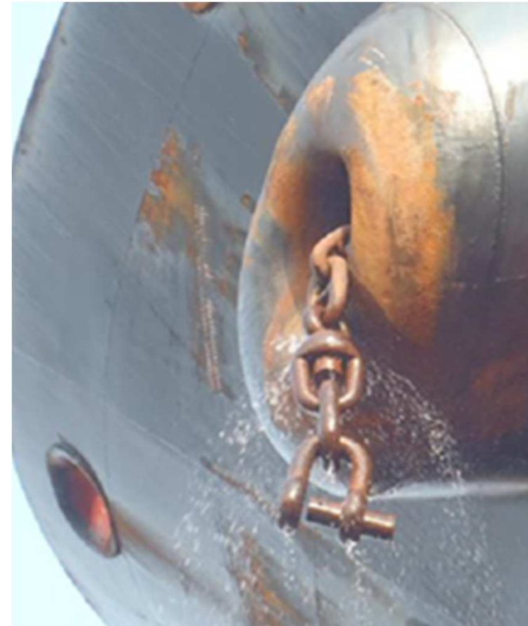
Anchor lost due to D-link opening up
