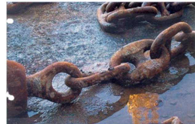
Heavily worn and bent anchor chain links
