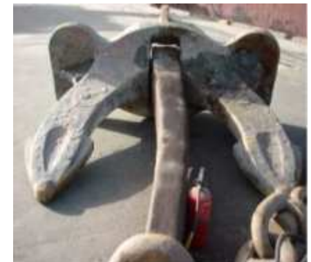
Bent anchor shank may be straightened
