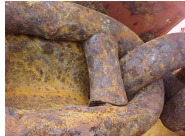
Loose and dis-located studs
