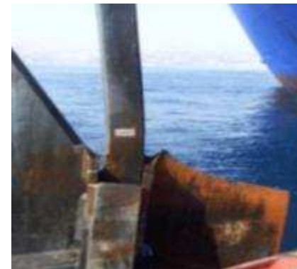
Anchor shank bent, fluke broken
