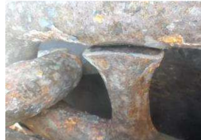
Stud with excessive gap
