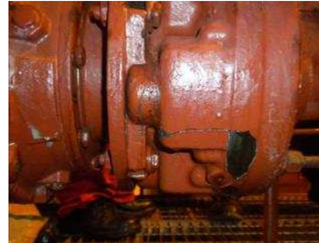
Hydraulic motor exploded during heaving anchor in heavy weather
