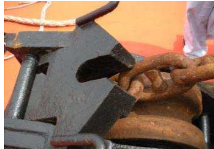
The pawl does not fit the chain
