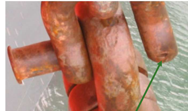
D-link bolt almost lost due to missing securing pin
