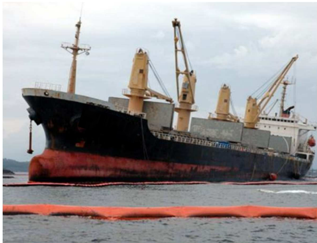
Vessel grounded due to dragging of anchor
