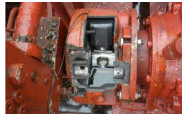
Hydraulic motor with broken cover plate
