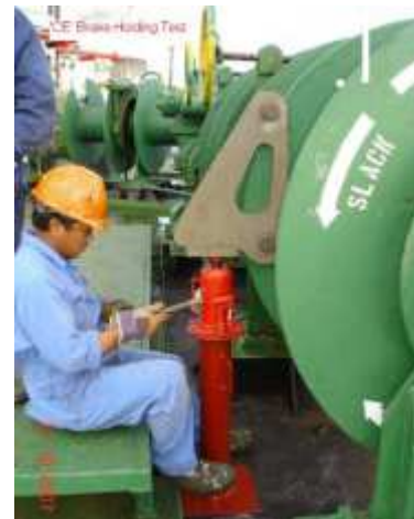
Brake band jack up test
