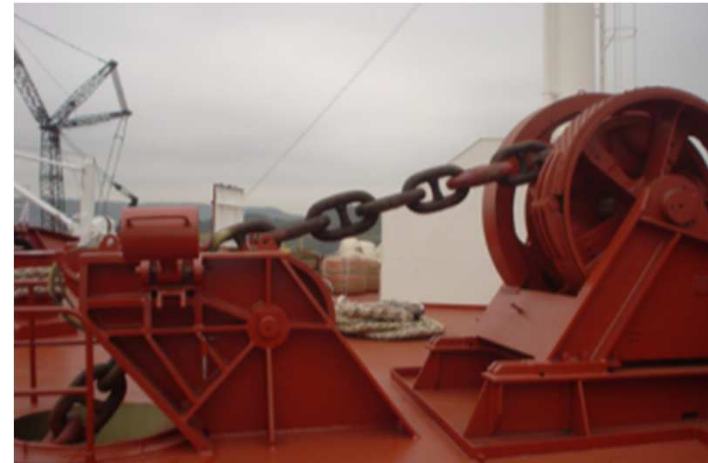
Conventional chain stopper arrangement
