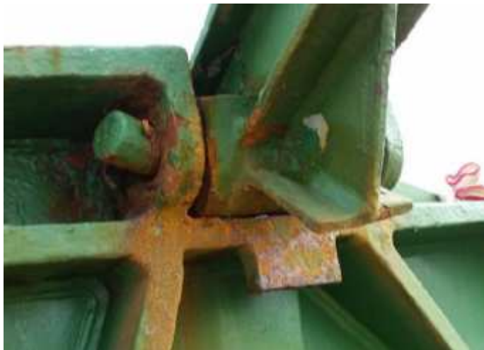
Chain stopper hinge pin severely deformed Ungraued
