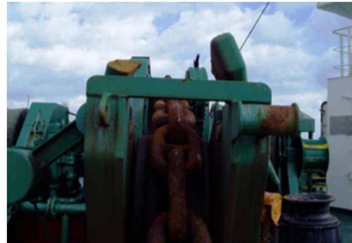
Guillotine bar broken
