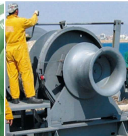
Applying the brakes while lowering the anchor
