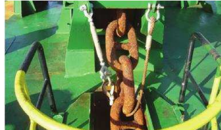
Securing of chain by turnbuckles (©OCIMF )
