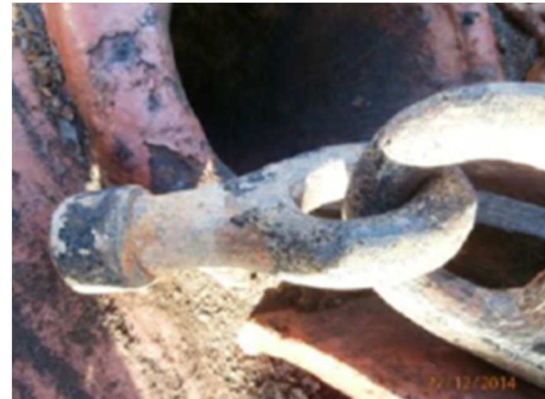
Anchor lost due to detached eyelet axle pin
