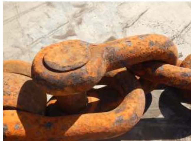
Remember to check the taper pin on opposite side !
