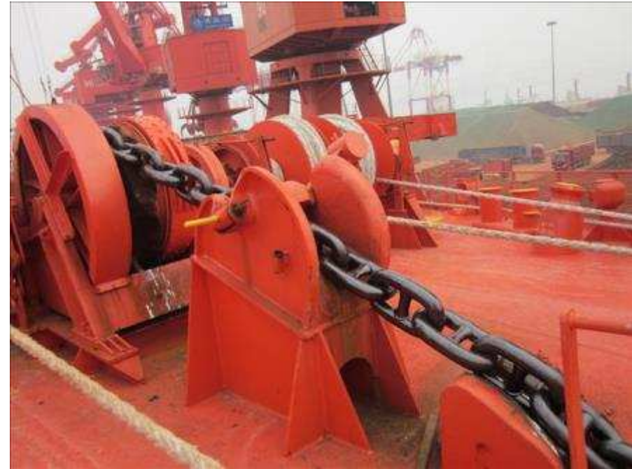
Windlass and chain stopper with guillotine bar
