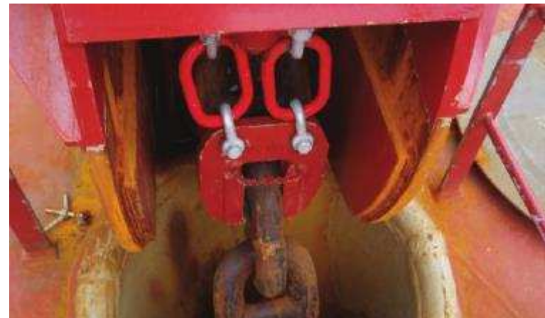
Securing of chain by Devils Claw(source ©OCIMF )
