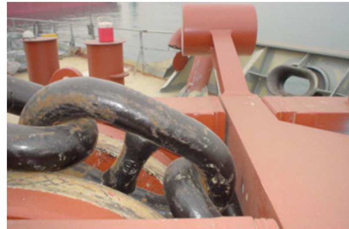
Guillotine bar engaged
