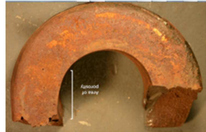
Broken anchor shank due to brittle material
