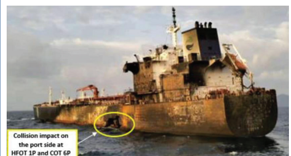
Damage to the vessel underway after collision and fire
