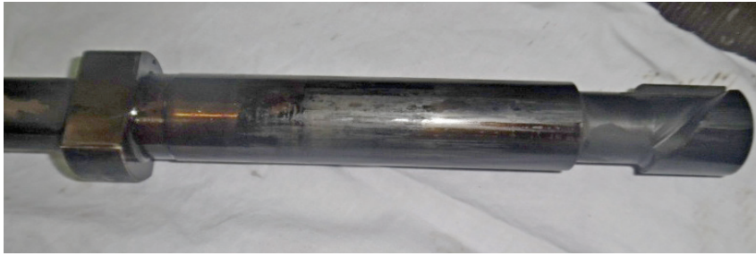
Fuel injection pump – the plunger was found completely seized in the barrel
