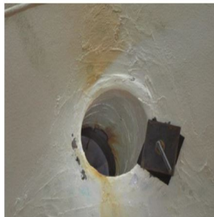
Temporary repairs on hull performed by diver on another vessel
