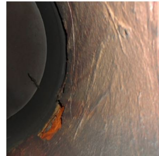
Protective coating inside disch. pipe flaking off at flange
