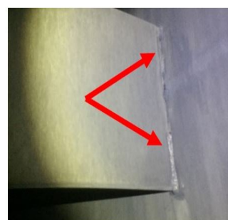
Poor workmanship: Support plates only spot welded by yard
