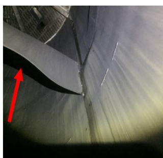
Deformed plates and buckled scrubber housing
