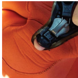
Bottom of zipper failure due to glue separation
