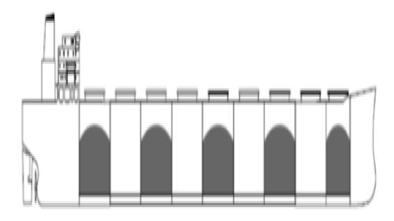
Alternative Hold Loading Condition (Fully Loaded) extracted from the IACS document Rec46
