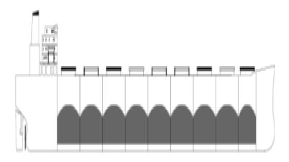
Homogeneous Hold Loading Condition (Fully Loaded) extracted from the IACS document Rec46
