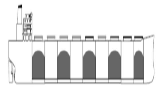
Alternative Hold Loading Condition (Fully Loaded) extracted from <u>the IACS</u> <u>document Rec46</u>
