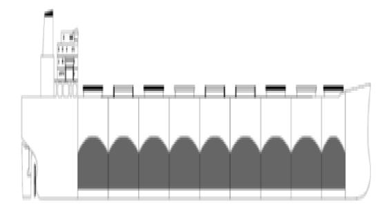
Homogeneous Hold Loading Condition (Fully Loaded) extracted from <u>the IACS</u> document Rec46
