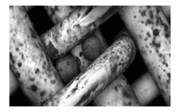
Catfines are extremely hard and abrasive. They can scratch or become embedded in the steel surfaces of marine engine components, particularly those that move against each other. When they enter an engine, they can lead to high wear rates and scuffing, resulting in costly damage to key parts. Factors like a vessel's motion in rough seas can stir up previously settled material in fuel tanks.
