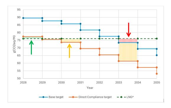
Fig.2 Illustration of Compliance Surplus, Tier 1 and Tier 2 Compliance Deficits based on LNG
