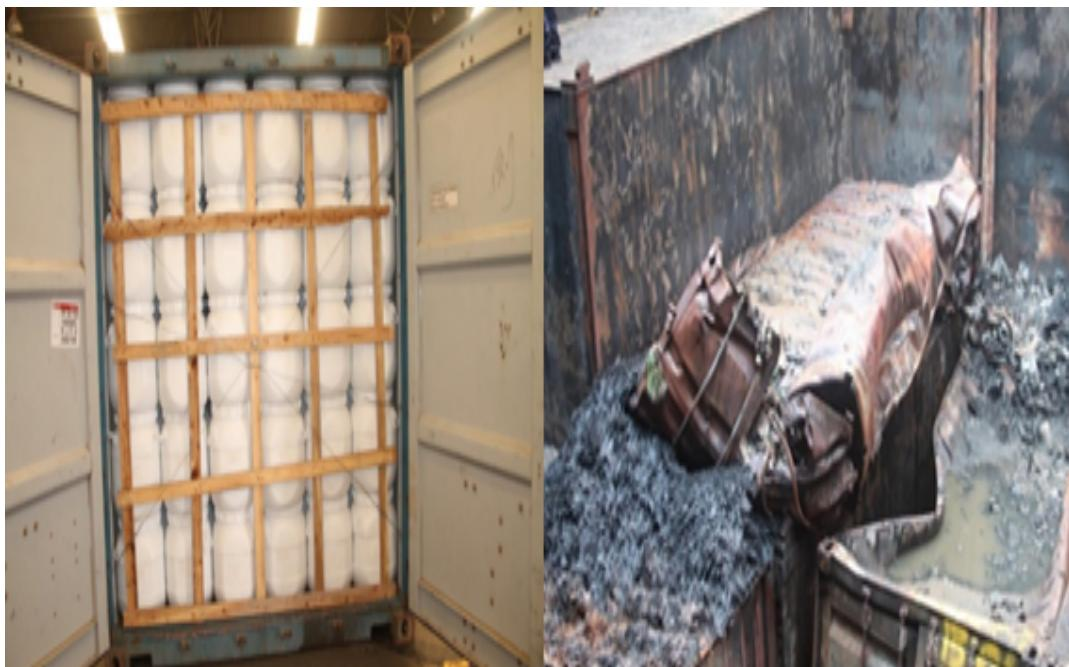
*A shipment of calcium hypochlorite with no room left for heat to escape – with inevitable consequences*
