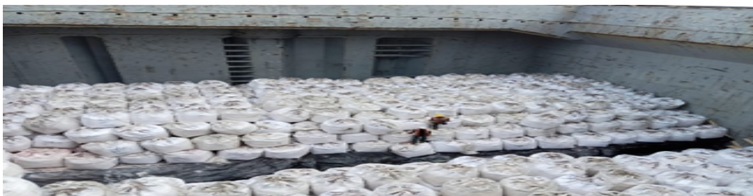
Bagged chemical cargo loaded above steel cargo
