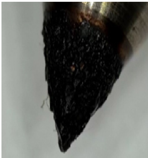
AE injector needle with sticky deposits
