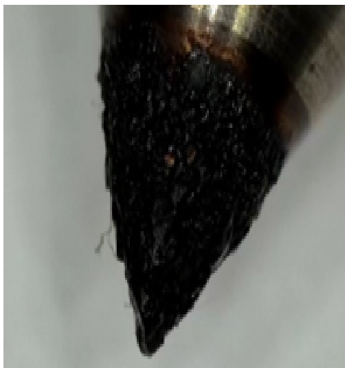
AE injector needle with sticky deposits
