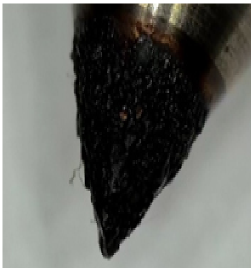
AE injector needle with sticky deposits
