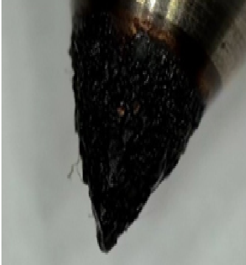
AE injector needle with sticky deposits
