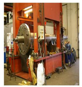
A bent propellar shaft 1 meter out of line, and after repair.
