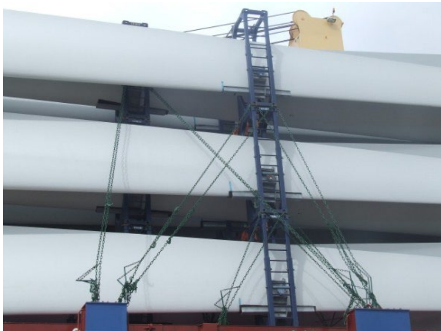
Chains securing Windmill Blades tensioned and hooked to D-rings welded on deck structures
