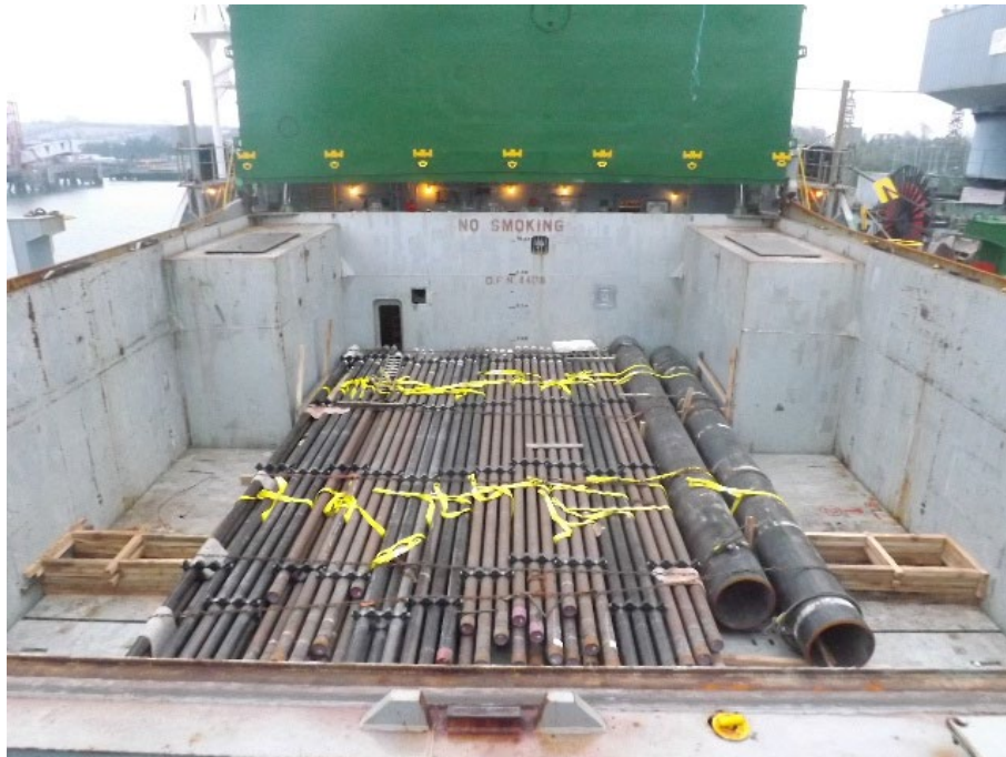
Steel pipes lashed with chains positioned athwartship and braced with softwood timber
