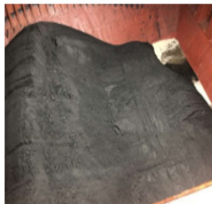
Cargo surface flattened and water accumulation noticed a day later
