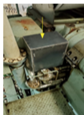
Guard fabricated to cover fuel system buffer (damping) tank
