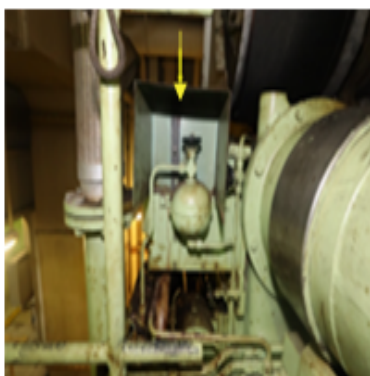
Spray shield around the pressure damper on auxiliary engine
