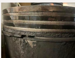
Piston rings broken and build up of carbon on cylinders
