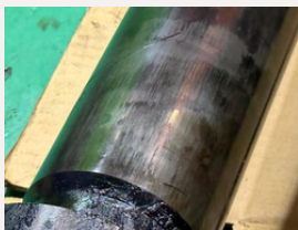
Wear and scratches on plunger
