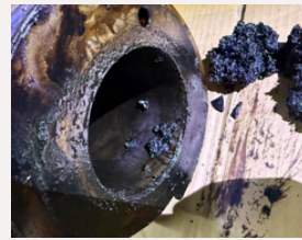
Sediment in fuel pump housing
