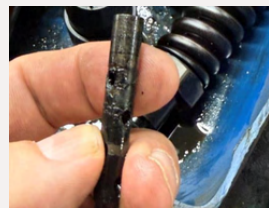
Injector tip showing signs of carbonization
