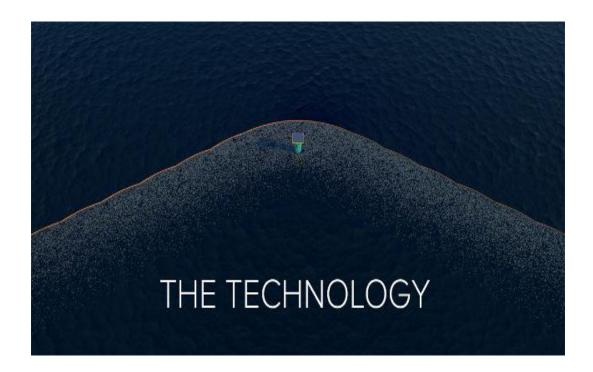
Slat has other ideas. Instead of going after the plastic using boats and nets, The Ocean Cleanup Array, a series of long floating barriers, uses the natural movement of the ocean currents to passively collect plastic in front of the booms. The plastic can then be removed and collected by ship for recycling. By using booms rather than nets the possibility of catching and harming marine life (by-catch) is sigificantly reduced.
