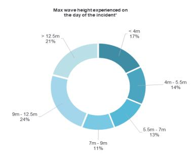
\*This chart shows the maximum wave height experienced by the vessels on the day of the incident, whereas the previous graph showed the average of the maximum wave heights to which the vessels were exposed over a 7-day span. Source: Gard
