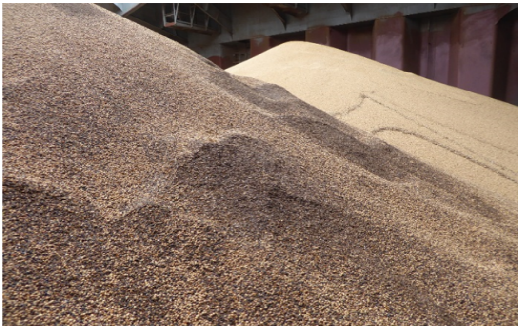
PHOTO 3: Small lumps of heat damaged soya beans dispersed sporadically throughout the cargo is consistent with the soya beans having undergone self-heating prior to loading or 'bin-burn'.
