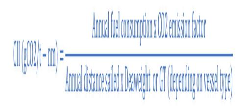
As the formula stands currently, calculation of carbon intensity is based on the consumption of fuel and its fixed carbon factor, and not on direct measurements of the emissions at the engine exhaust side. Also, there is no benefit given for carbon capture onboard. A lower numerator and/or a greater denominator can result in lower carbon intensity. Focusing on the numerator first, the following factors can have a positive impact on the CII rating for a given calendar year:
