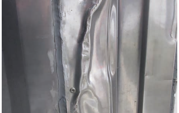
Picture 7 Cargo damage to the stainless steel side lining.
