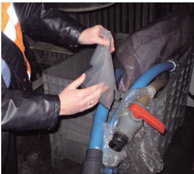
Example of a five-ply plastic flexi-tank.
