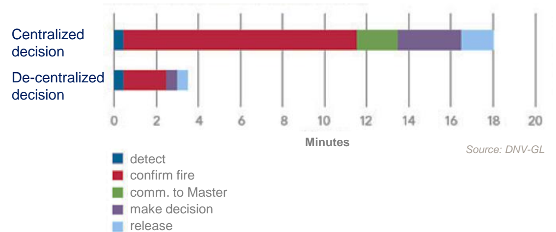
REACTION TIME – WATER SPRAY FOR RO-RO DECKS
