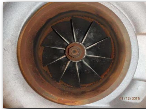
Chloride affected corrosion in auxiliary engine turbocharger.
